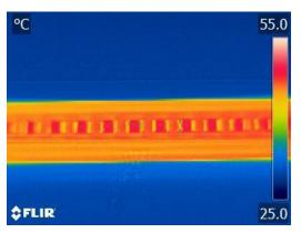
Figure 4. Thermal Distribution in the LED Tube
