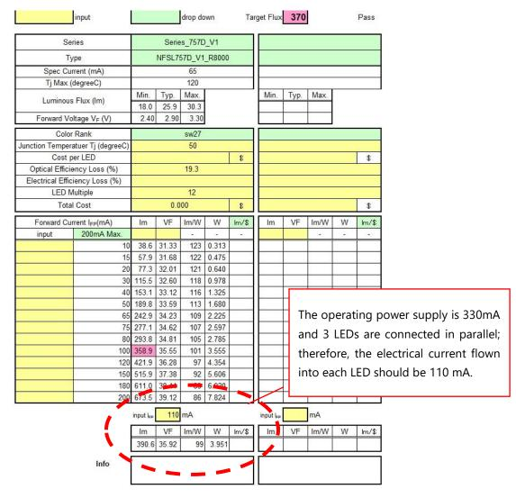
Figure 7. Example of Calculation (LED Down Light)
