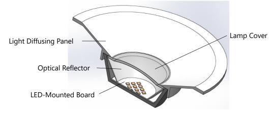
Figure 6. LED Tube Structure
